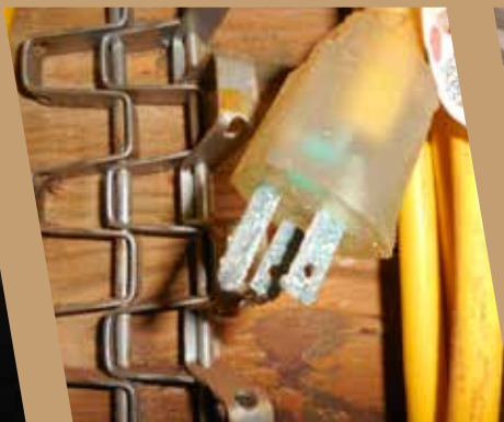
Corroded light fixture and electric plug demonstrate the corrosive nature of dry fertilizers; the mislabeled bin of red potash can lead to application errors.
